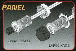
To panel mount your PLC-U, find a flat panel and drill a 1" (25mm) hole. You have the choice of using either the small or large knob with their corresponding bezel.
