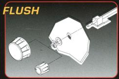
For a flush mount application, you can remove the attenuator from the rocker switch mount. Drill a hole for the attenuator to pass through, use the retaining nut a washer to secure and slide on the knob of your choice.
