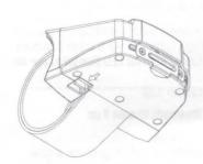
To release the remote from the steering wheel mount, push the tab on the underside of the unit in the direction the arrow is pointing. While holding the tab, pull the unit straight up and out of the mount. If the unit is going to be used standalone and not fixed, included is a flat cover that slides on to the unit making it a mobile remote.
