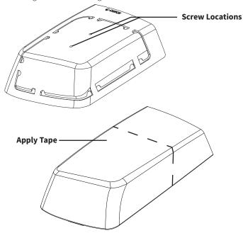
Step 3. Apply the template to the saddlebag lid and secure using (2) screws that came with the kit.
