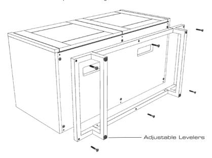
C. Secure tube base with washers and screws.
