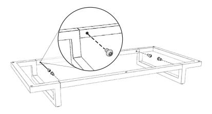
**B.** Attach tube base to your cabinet using connector bolt.
