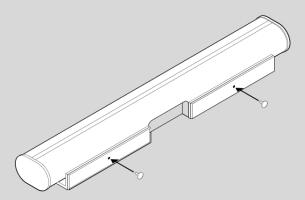
5. Screw the 2 knobs into the back of the soundbar until they are fully tightened.
