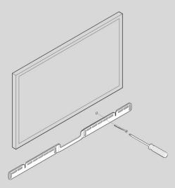
**4.** Position the wall mount bracket over the marked screw locations, using a level to confirm accuracy. Use a Phillips-head screwdriver or a power drill to screw the bracket to the wall, making sure the arrows in the center are pointing up.
