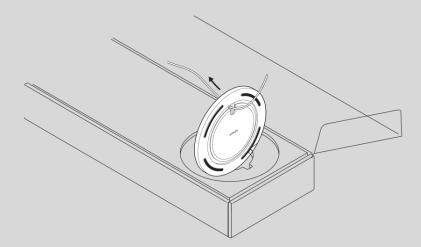
2. Insert the stem snugly into the base, using the alignment pins to position the power cord channel either in the front or back. Use the 2 black screws and a Phillips-head screwdriver to attach the base.
