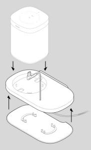
7. Wrap the excess power cord around the bottom of the shelf.
