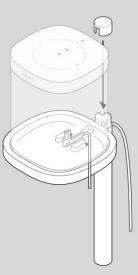
**6.** Press the power cord into the stem, working from top to bottom. Pull the excess cable down from the base.
