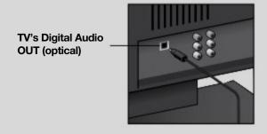
IMPORTANT: Remove the protective caps from each end of the optical audio cable before inserting.
