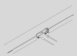
6. Connect the power and HDMI cables to the back of the soundbar.
