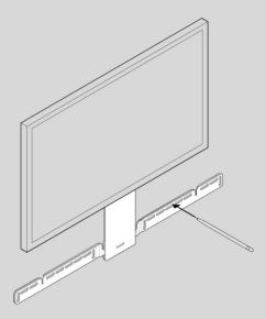
2. Mark the screw locations and remove the guide. Refer to Wall mounting information for placement help.
