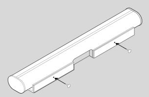
5. Screw the 2 knobs into the back of the soundbar until they are fully tightened.
