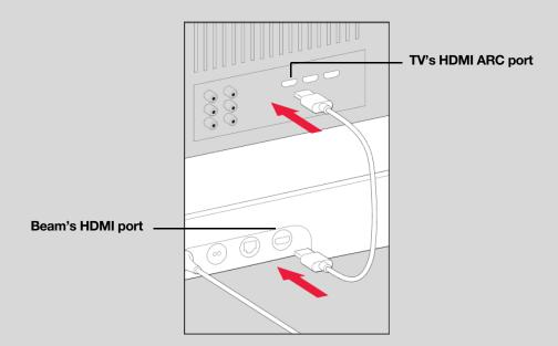
**Note:** If you can't find the word "ARC" on the label, it isn't the correct port. See **If your TV doesn't have an HDMI ARC port**.
