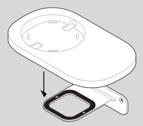
5. Route the speaker's power cord through the shelf opening. (You'll wrap the cord around the bottom of the shelf after it's assembled.)
