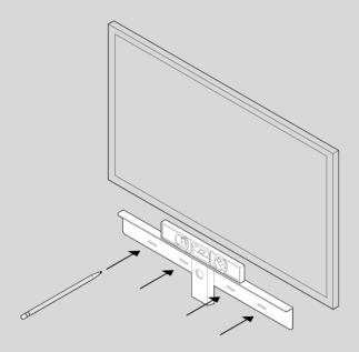
3. Use a 5/16" drill bit to drill pilot holes (see Wall mounting information)
