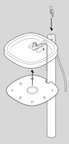
5. Plug the power cord back into the speaker and place on the top mount, pulling any extra cable down from the top. Tighten the screws and attach the top cap with the notch facing toward the speaker.
