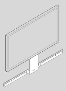
1. If your TV is wall-mounted, place the positioning guide against the wall, aligning the top edge with the bottom of your TV. There should be 5.5" (140 mm) between the top of the wall mount bracket and the TV.
