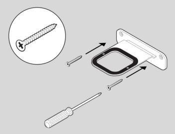
4. Position the shelf the way you want it (supports left or right speaker placement). Press the shelf firmly on to the wall bracket until it snaps into place (both front and back).
