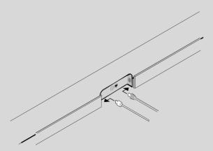
6. Connect the power and HDMI cables to the back of the soundbar.
