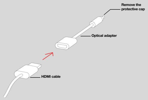
3. Connect the optical adapter to the TV's optical digital OUT port.
