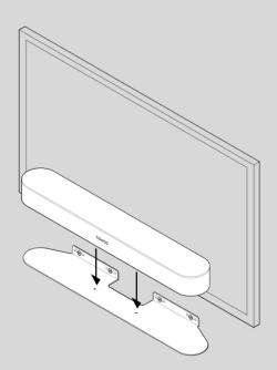
8. Insert and tighten Beam to the bracket using the mounting screws.
