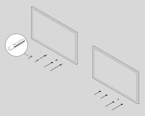
5. Place the bracket on the wall and loosely tighten the wall screws to secure the bracket. Check with a level and then tighten the screws.
