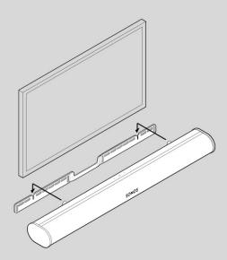
7. Slide the soundbar down so the knobs fit into the slots on the wall bracket. Make sure the touch controls are facing up, and the soundbar is fully seated.
