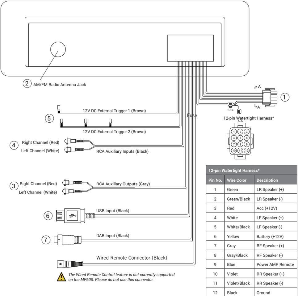
**⚠️** No lower than a 2 Ohm speaker load should be used or damage may occur to the stereo. Make sure the polarity of speakers is connected correctly.
