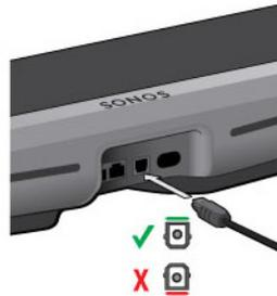
*The PLAYBAR's digital audio in and the optical cable end are 'D-shaped'—be sure to align for proper insertion.*
